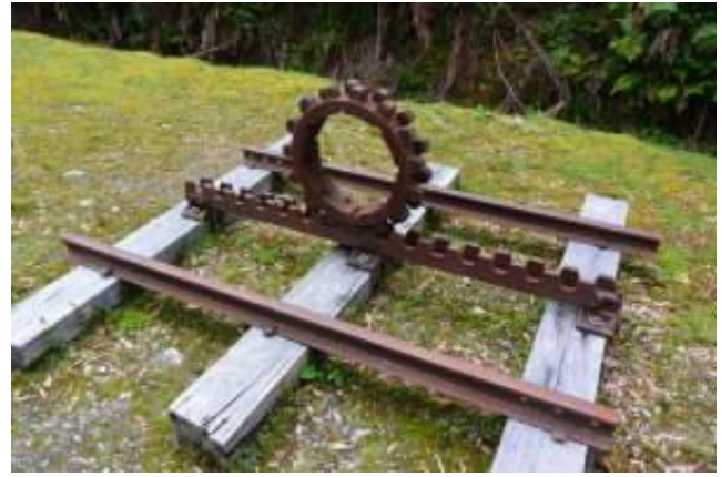
The Abt rack and pinion system
