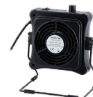
EXHAUST FAN / FUME EXTRACTOR - ADJUSTABLE Code: SOLDFFANADJ The practical solder fume extractor with different speed settings can not only be used as a table fan but also on a beam can be mounted. You have the choice, which positioning option you prefer. Piece of carbon filter is included. Air flow-rate: -1.2 m³/min Max. noise generation 45 dBa Dim(L x W x H): 185 x 135 x 217 mm Max. power: 23 W Operating voltage: 230 V AC Absorption capacity: 0.2 to 1m3 / minute. $60.00
