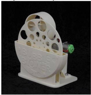
Printing time for the quality that I used was really huge - probably a couple of days, not including reprints etc The wall thicknesses that I use are typically 2.4mm, which means that there are 2.4m/0.4mm(print width) = 6 passes of the nozzle.
