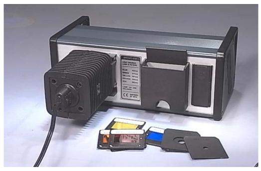
The image above shows the lamp mounted and the filters and apertures on the bench. They are normally stored in the container mounted to the panel. A small label lists the shortest wavelength (highest frequency) of light that can pass through each filter.
