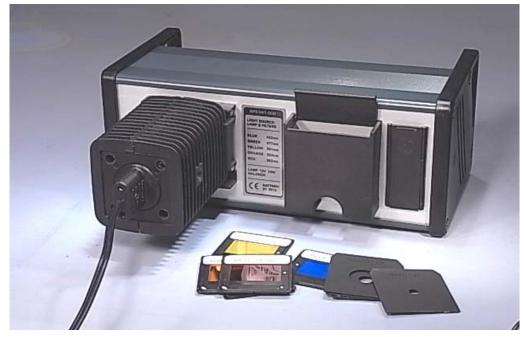
The image above shows the lamp mounted and the filters and apertures on the bench. They are normally stored in the container mounted to the panel. A small label lists the shortest wavelength (highest frequency) of light that can pass through each filter.
