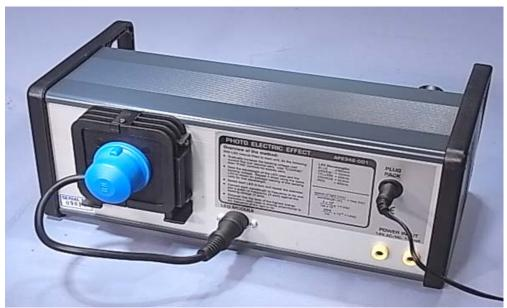
The image above shows the LED panel positioned correctly and plugged into the instrument. The 12V.AC or DC PlugPak socket and the 4mm banana sockets are on the right side.
