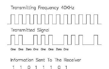
Using this method of information it is possible to have 256 different commands. The controller with this kit has only 4 commands to allow you to control the forward and reverse operation of 2 different motors.
