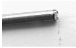
Deformed end of cut shaft.
