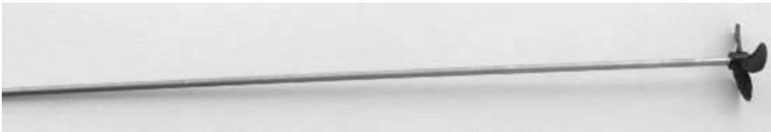
Propeller fitted to shaft.
