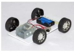
This project requires the student to design and build a *SIMPLE VEHICLE*. This is the most basic vehicle possible, and is suitable to introduce students to Technology and Electrical components. After completion of the vehicle, it can be used for a variety of experiments (physics or otherwise) or even paired with another vehicle for racing and performance tests.
