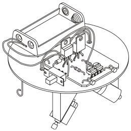
If light is shone onto both sensors the robot will move forward in a straight line. By using a torch as the light source the robot can be steered.
