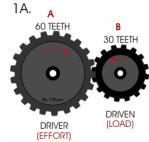
$= \frac{1}{2} = \frac{\text{Input movement}}{\text{Output movement}}$
