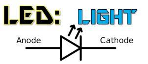
The <u>light-emitting diode</u> (LED) is an versatile piece of technology that has revolutionised the way we use lighting. LED light is a solid state light as there are no gases, no filaments and no moving parts to fatigue.
