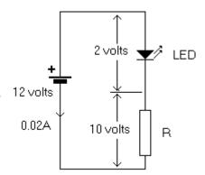
To calculate the value of the series resistor we need to know the diode forward voltage and current and its
