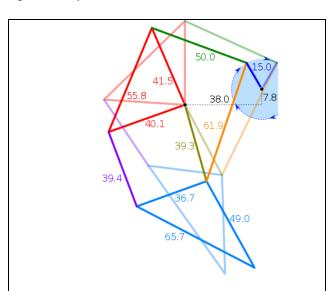
"Theo Jansen's linkage. When the blue line at the right end of the picture is driven in a clockwise rotary motion, the leg (blue triangle at the bottom) executes a walking motion.
