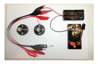
Kit includes switch, bulb holder, bulb, battery holder, alligator clips, tape and screws. This kit is designed to be used by groups of 2-3.
