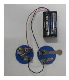
With the Switch closed electricity flows to the light
