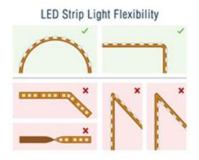
A LED strip light is a flexible circuit board that is populated with LEDs allowing it to be mounted on curved and uneven surfaces. They can bend up or down but not on its horizontal axis (left or right). They have the advantage of being longer lasting and energy efficient.
