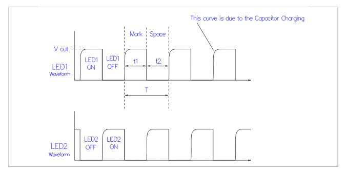
The circuit alternates between one state in which transistor T1 is "OFF" and transistor T2 is "ON", and a second state where T1 is "ON" and T2 is "OFF".
