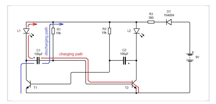
As the capacitors charge one of them will charge slightly faster and reach the voltage needed (0.7 volts) at the base of one of the transistors to turn it on.
