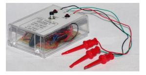
The *TRANSISTOR TESTER* described here will indicate whether a suspect transistor is good or faulty and, as a bonus, tell you the component's type (PNP or NPN).
